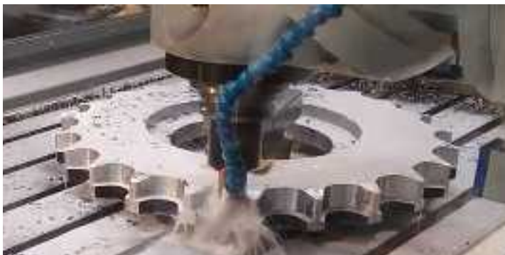
Cat Track Sprocket: Profile Full CNC machined in one operation using CAD/CAM technology
