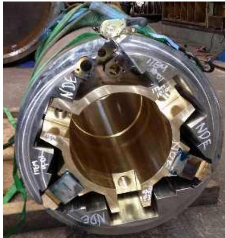
Steel Coil Expanding Mandrel: Complete new manufactured and fitted in house to exacting tolerances.
