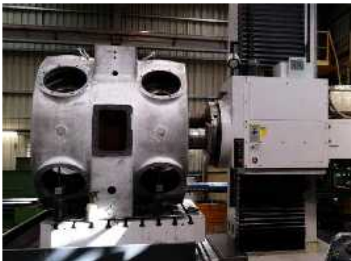
800mm Dia Compressor Body: Bored and ported true
