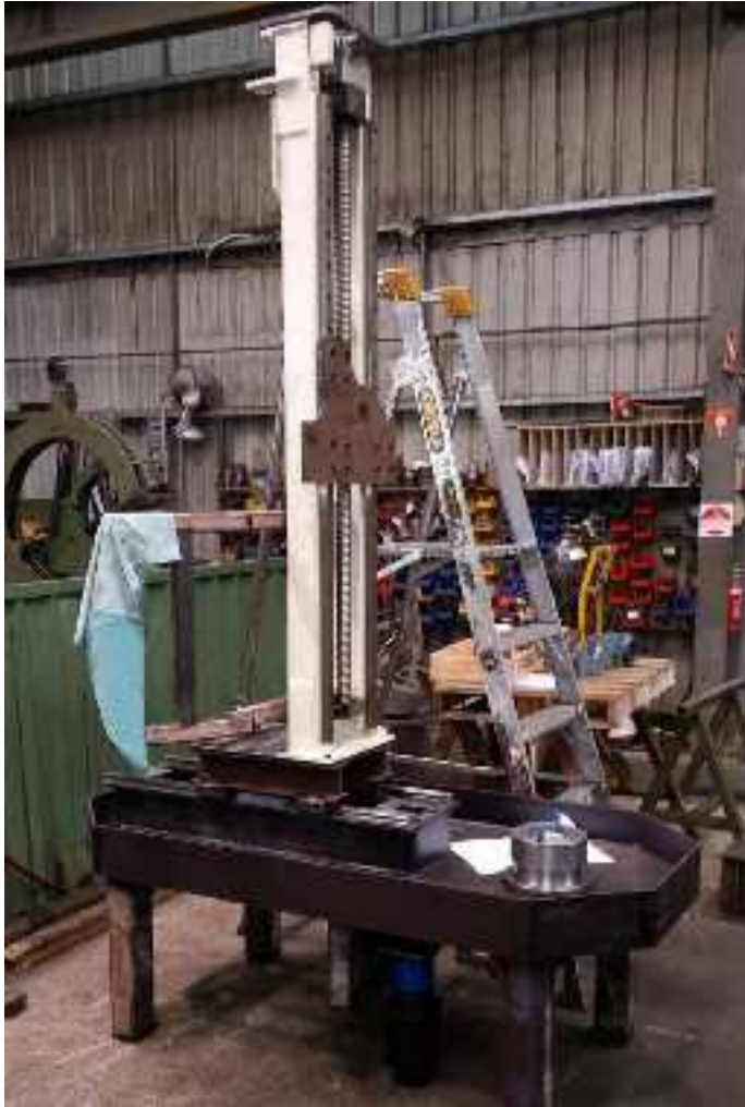
CNC Flame Hardening Machine: Manufactured and assembled in house complete with all mechanical and electrical components.
