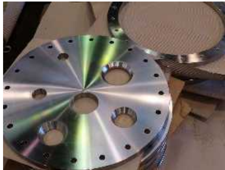
950 Dia SS316 Flanges: Turned and drilled through
