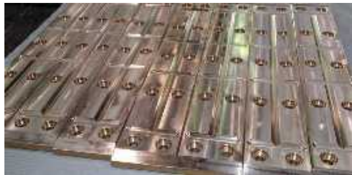
Bronze Wear Pads: Machined complete from bronze castings
