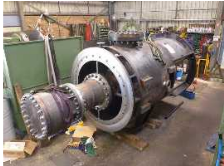
1800mm Dia Steam Discharge Head: Fabricated and machined complete
