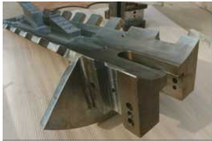
4 Expanding Mandrel Segments: Machined from a 4140 Billet - 1200mm X 500mm X 350mm
