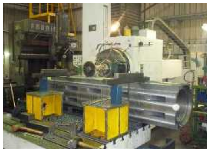
Mandrel Sleeve: Machined complete from cast iron
