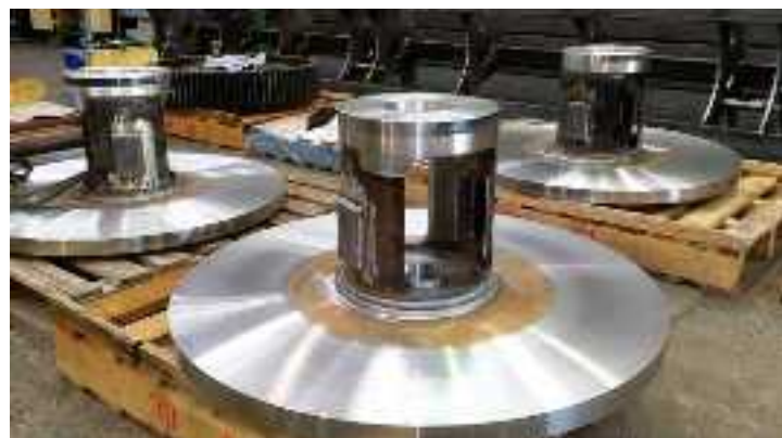
Valve Yokes: Fabricated and machined complete
