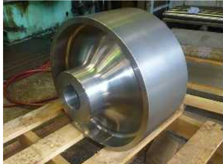
19" Diameter Brake Drum: machined from a solid billet of K1045
