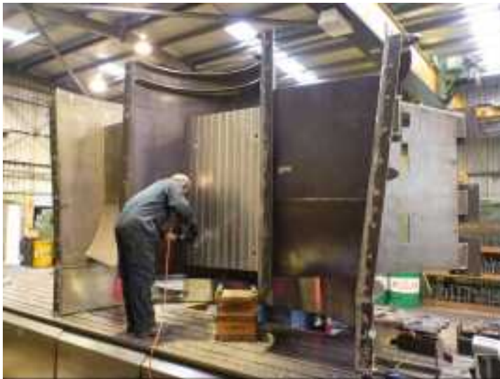
Fan Base and Duct: Machine the mounting plate
