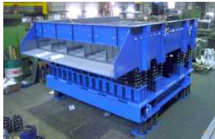
Large Shaker: Fabricated and machined complete in house
