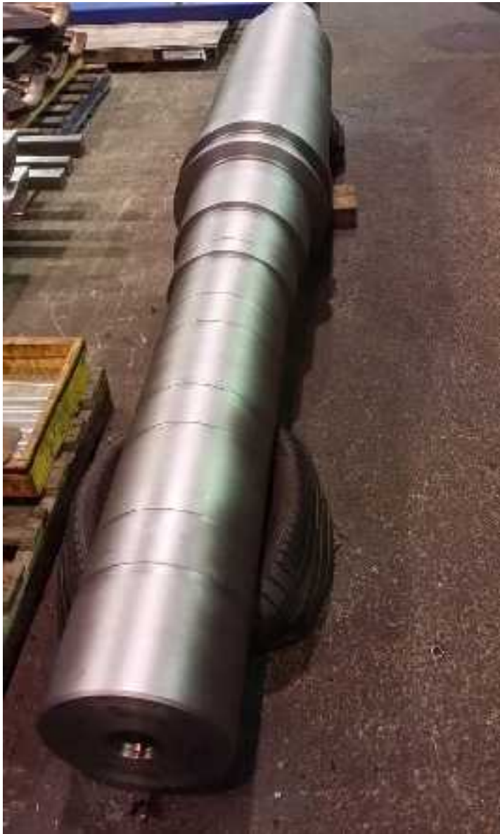
4m Mandrel Shaft: Machined from a 7 tonne solid forging down to 4 tonne
