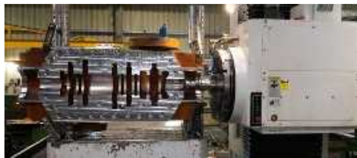
Multi-Stage High Pressure Centrifugal Pump Body: Faced, drilled and bored.
