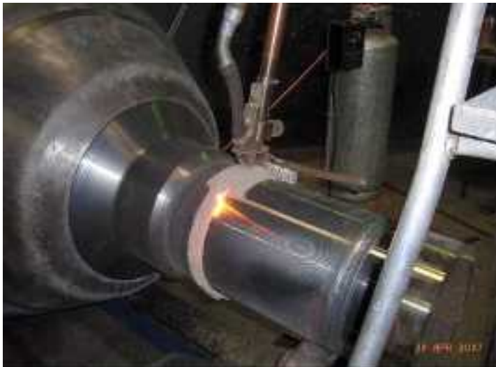
Shaft Journal Rebuilding: Sub-Arc and MIG lathe welding for building up shaft journals - remachining in house
