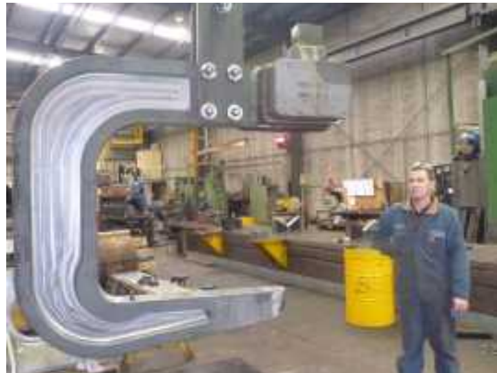
30t WLL "C" Hook: Over 1,000 kgs of material was removed from the main 200mm thick body
