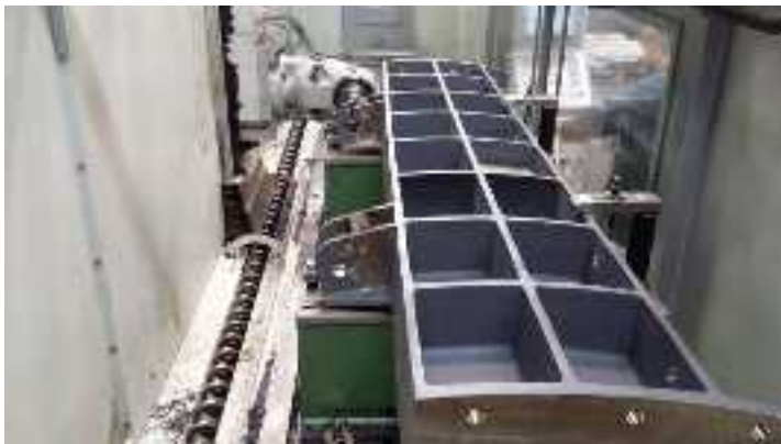
4 Off Arc Gates: Manganese Steel machined on faces, drilled and bored.
