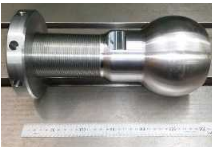
Ball Joint: CNC turned with fine thread and nut
