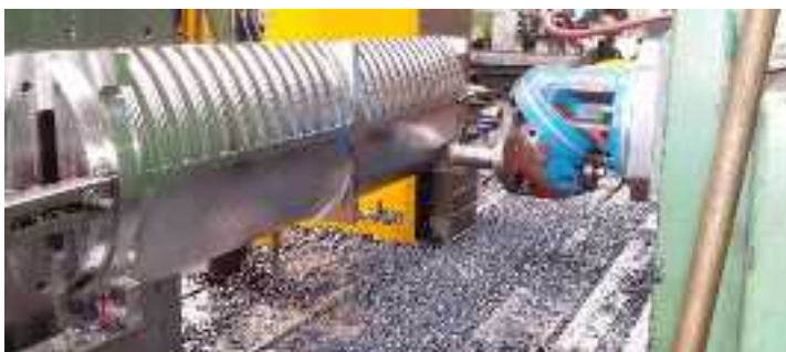
3 off Mandrel Segments: Manufactured complete from a solid 4340 forging.
